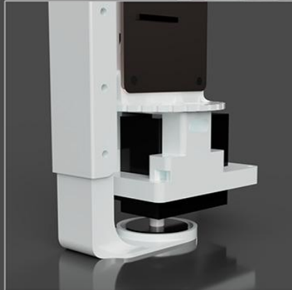
Magnetically coupled servo bracket
